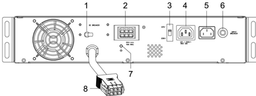
1. The DC Breaker connects and disconnects the DC bus voltage from the Battery Pack to the UPS. The DC Breaker will trip in the event of a DC overcurrent condition.
