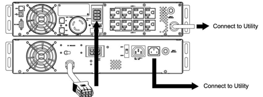
**NOTE:** The BP72RTXL's External Battery Cable has a strain relief that must be attached (with the screw) to the rear panel of the UPS.
