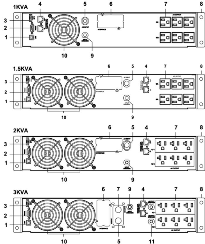
1. The USB Communications Port is for UPS monitoring and control.
