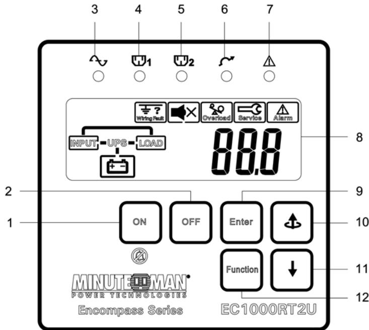
1. The ON button is to turn the UPS on. Pressing the ON button during the Battery mode will silence the alarm.
