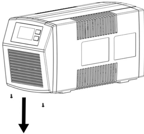
7. Slide the front panel downward, then outward, and then move to the side or lay it on the top of the unit. (FIG. 2)
