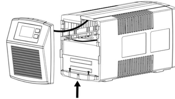
12. Grasp the battery pull tab and gently pull the battery module out of the UPS and set aside. (FIG. 3)
