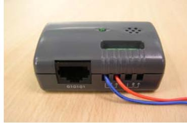
3. Connect the straight-through CAT5 network cable from the SNMP-SSL card's RJ45 connector labeled "COM" to the connector labeled "010101" on the SSL-EMD.
