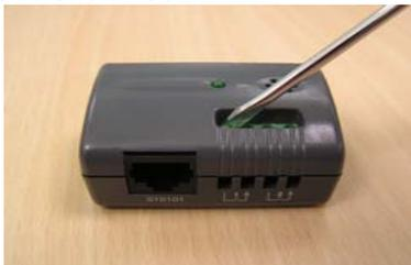
2. Connect the wires from the SSL-SMOKE detector to the SSL-EMD Alarm-1 and/or Alarm-2, and then tighten the screws.
