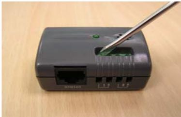
2. Connect the wires of SSL-VIBRATION sensor to the SSL-EMD Alarm-1 and/or Alarm-2, and then tighten the screws.
