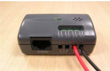
3. Connect the straight-through CAT5 network cable from the SNMP-SSL card's RJ45 connector labeled "COM" to the connector labeled "010101" on the SSL-EMD.
