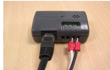
4. Verify that the SNMP-SSL card has a network connection and is powered on.
