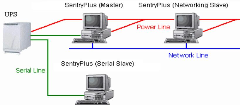
If there is a communication cable between the computer and a UPS, this computer called Master. The Master can monitor and control the connected UPS directly, as it also transmits the UPS information to the Slave(s).
