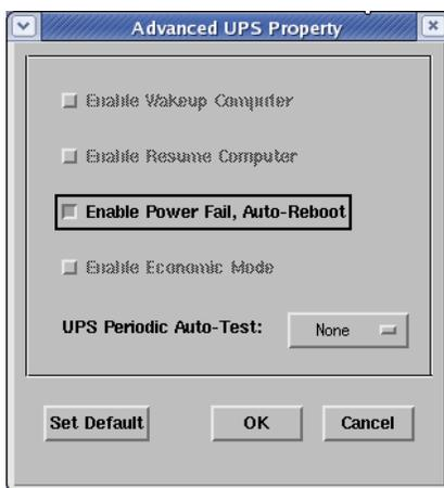
**Enable Wakeup Computer:** If your computer's architecture is compatible to ATX and the BIOS supports RS-232 (RI) Wakeup function. You should enable this item to make the Schedule work correctly.
