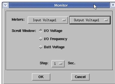
**a. Meters:** Press the Main button in the Bottom Layer Buttons there are two meters in the information area. You can change the display items of the two meters.
