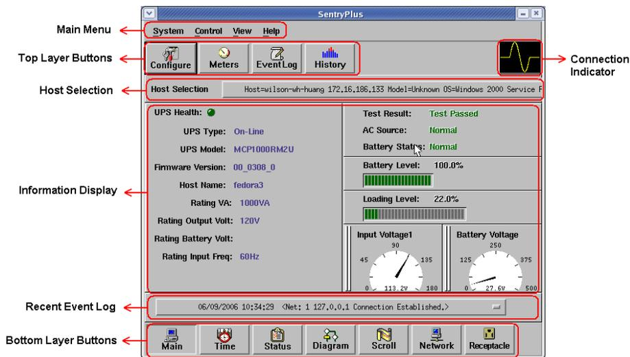
**Host Selection:** Press the combo box to select hosts that runs SentryPlus Service in the LAN. Users can monitor or control (need password) remote UPS.
