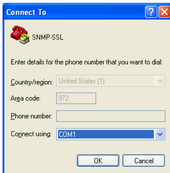
Figure 2-5: Select Direct to COM port connection
