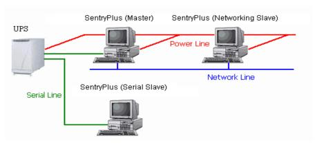
If there is a communication cable between the computer and a UPS, this computer called Master. The Master can monitor and control the connected UPS directly, as it also transmits the UPS information to the Slave(s).
