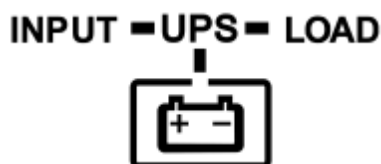
Battery Mode Power Flow
