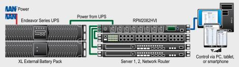
Utilize a Minuteman RPM unit in conjunction with a UPS to ensure fail-safe, controllable power. In this example, conditioned and backed up power from the UPS is provided to multiple servers and a router from the RPM2082HVI.
